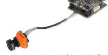
Always press and pull on the actual connectors during assembly or disassembly, never pull on the wires to remove a connector.
